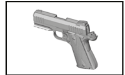
Fig. 1: Grip safety is activated
