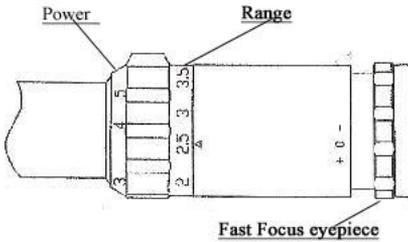
Hold the scope about three or four inches from your eye and look through the eyepiece at a featureless, flatly lit bright area such as a wall or open sky. If the reticle is not sharply defined instantly, you need just to turn the quick focus eyepiece in or out for adjustment until the reticle appears in sharp focus.
