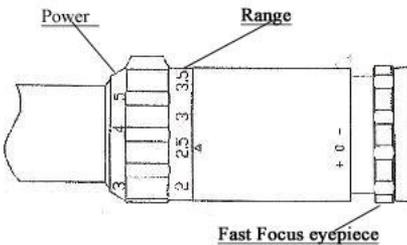
We call the new reticle the **No-Math Mil-Dot**, because you determine the range by just framing a meter, multiple meters or fraction of a meter of the target and then reading the range on the power change rings. This is much simpler than solving the above math equation. If you frame the target in meters then you read the range in
