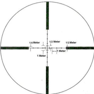
As you can see in Figure 1. There are numerous framing dimensions available on the reticle. Although not denoted, it should be clear that up to 8 meters in width or height could be used for framing. The total
