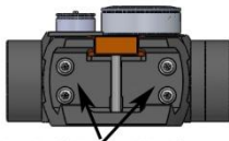
Four No. 10 Torx(Star)Head Screw
