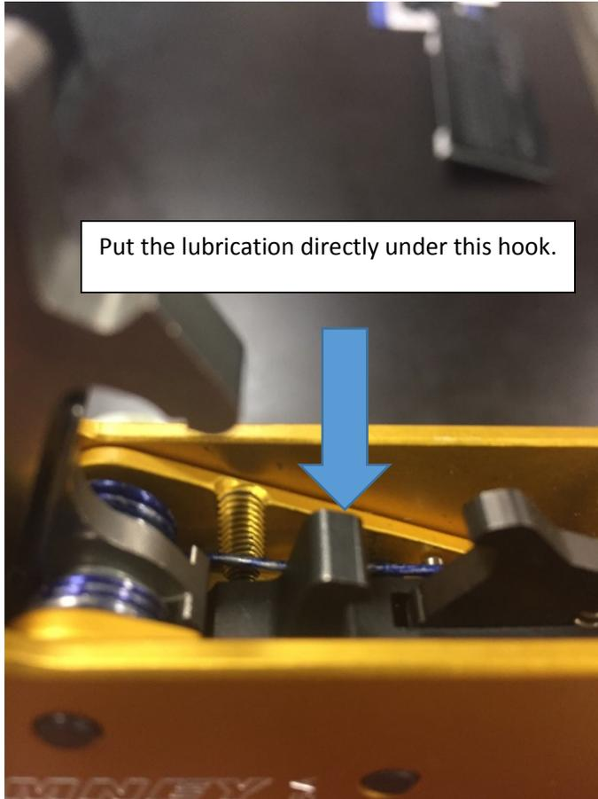
To reduce friction add grease to the underside of the hook.
