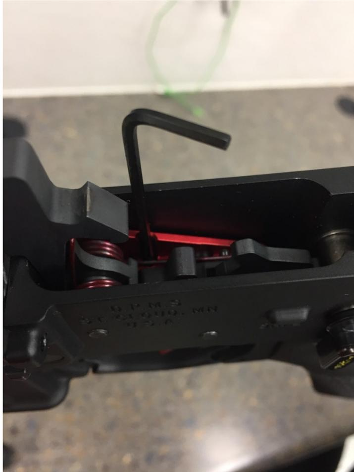
When installing your Timney Calvin Elite AR-15 trigger be sure to tighten down the set screws once the pins and safety are in place. No torque wrench is necessary, hand tightening should be sufficient.
